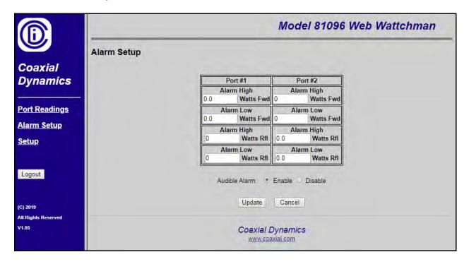
Model 81096 is equipped with an audible alarm. When a fault is detected and the system is tripped, the alarm will sound. Terminals 4, 5 and 6 will switch if either system one or two faults and can be used for an external alarm. These contacts are normally open and close during a fault condition. These contacts have a rating of 2 Amps at 115 VAC. The alarms are set using an Ethernet crossover cable.
